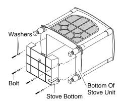
Figure 11 - Attaching Stove Bottom
